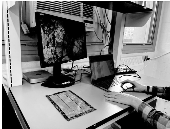
Fig. 5. An example of the 117cm 2 PDMS deployable film in triplicate within an indoor office space.
